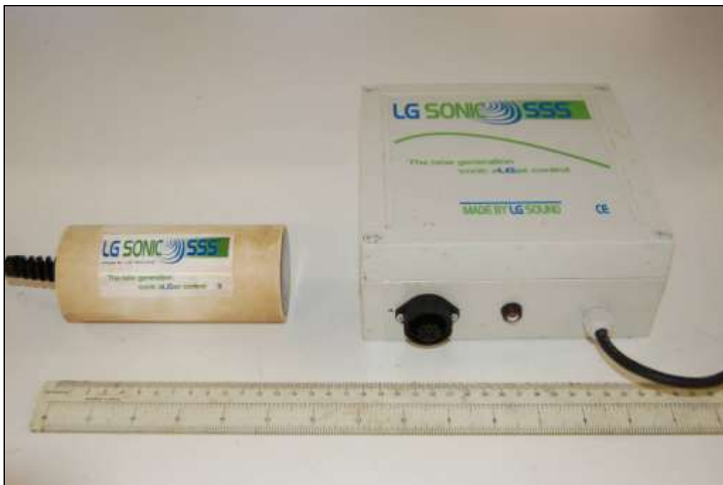
Figure 5: LG Sonic SSS ultrasound device, the cylindrical transducer is held horizontally below the water surface with the electronic box connected to a mains electricity supply.
